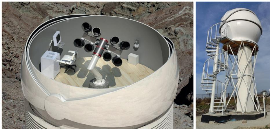
Figure 5: Left: the INF multiaperture telescope concept: 8×VT-78d tubes on ASA DDM160 mount. Right: the double-tube INF prototype is installed in the dome at Kislovodsk station of INASAN.
